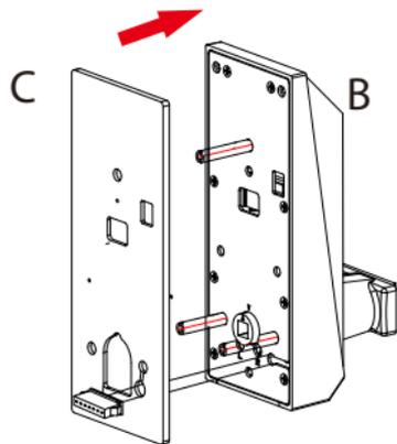
3.2 Insert spindle(H) into the clutch.
