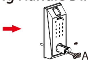
3. Insert mechanical key into hole to open the door.
