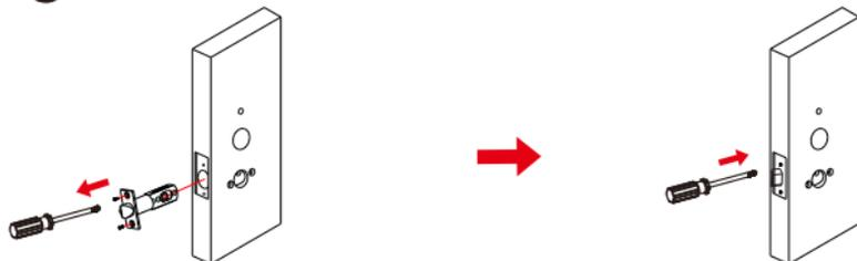
Remove screws from the latch trim panel with a screwdriver and rotate the latch bolt at 180°.
