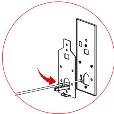
5.3 Secure indoor unit(K) to outdoor unit (B) by inserting screws(M) and screw(L).
