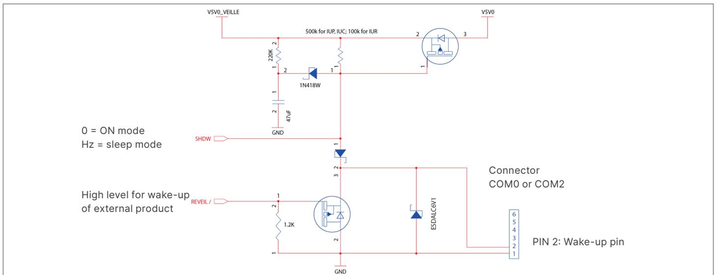
The wake-up pin must be high impedance. Do not connect directly any voltage on this pin even if the devices are 10V tolerant.
