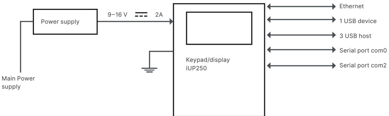
The terminal with its modules is centrally powered through the “Power” connector of the iUP250LE. The readers are powered through the USB Host connection.
