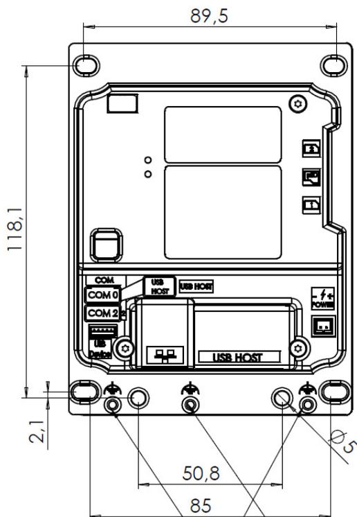
Autothread M3X8 for GND if central position not possible
