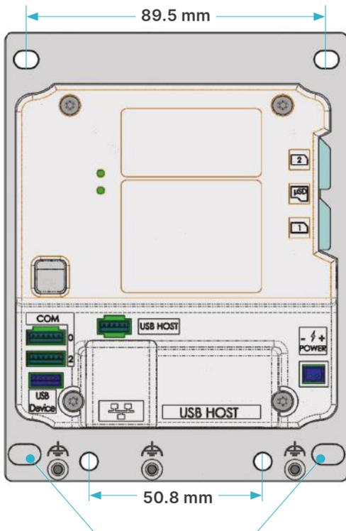
The outside "holes" on the bottom are not available for mounting! Please use the inner holes at a distance of 50.8 mm.
