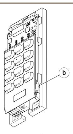
2. Check that the RS485 termination switch (b) is switched to ON.
