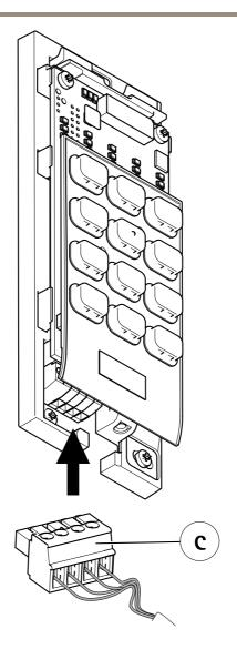
6. Reattach the connector head (c).
