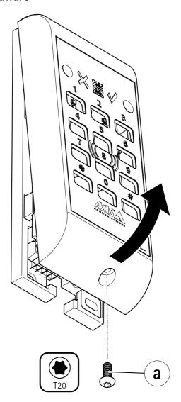
1. Remove the frontplate screw (a) and remove the frontplate from the reader backplate.
