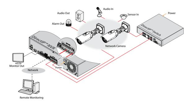
Directl $P^{TM}$  NVR makes it easy to use cameras without extra network configurations. Each camera can be controlled via the Directl $P^{TM}$  NVR setup menu, without any PC. For detailed camera settings, please see the camera setting pages of Directl $P^{TM}$  NVR manual.
