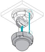
2 Fasten the screws for the dome cover clockwise using the allen wrench.
