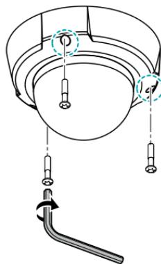
Attach the dome cover to the bottom cover. Press the area where the triangular mark meets the dome cover assembly hook to assemble the dome cover.
