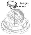
3 Use the screws, anchor provided with the camera to secure the bottom cover on a wall or a ceiling.
