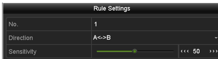
Figure 9.5 Set Line Crossing Detection Rules
