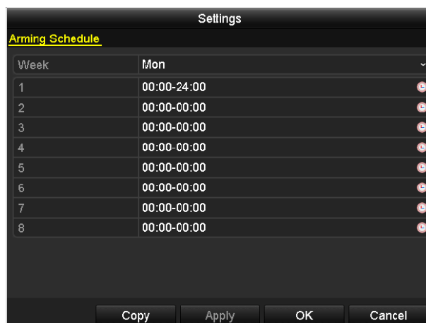
Figure 8. 16 Set Arming Schedule of Alarm Output
