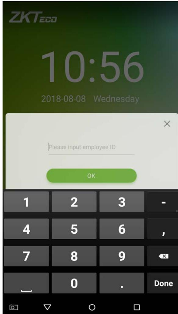
If an employee has registered a fingerprint and card in addition to a password and the verification method is set to fingerprint/password/card verification, the following screen will appear. Select the password icon
