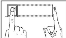
**Press your finger onto the fingerprint reader.**
