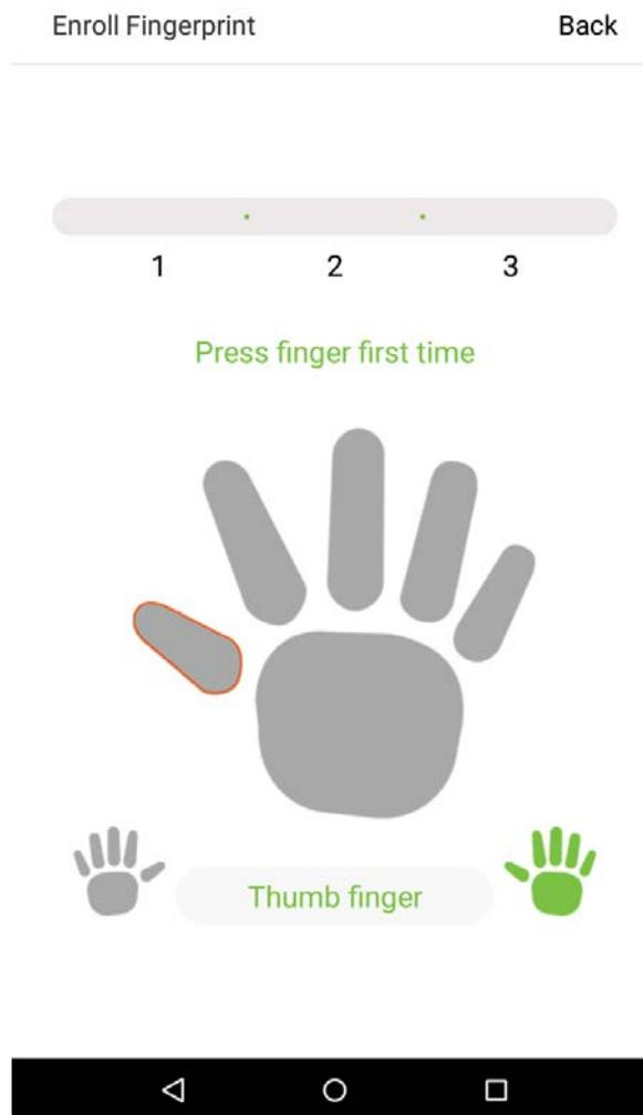
2. Press the same finger on the fingerprint reader three times. Green indicates that the fingerprint was input successfully.
