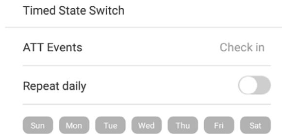
6. Tap on the button for the date you would like to set, then swipe up and down to set the corresponding time. Tap on [OK].
