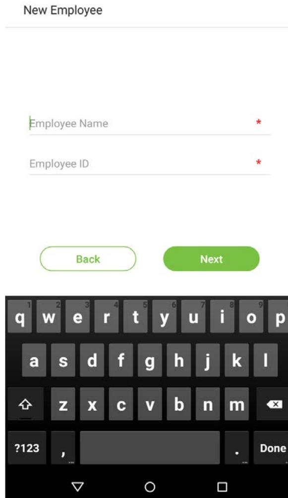
**Note:** This device supports input methods of Chinese, English, numbers, and symbols. Press [CN] to switch to the Chinese keyboard; press [EN] to switch to the English keyboard; press [?123] to switch to the numbers and symbols keyboard; and press [Back] to return to the alphabet keyboard. If you tap on an input box, the virtual keyboard will pop up on the screen. To hide the keyboard, tap on the downwards arrow ▾.
