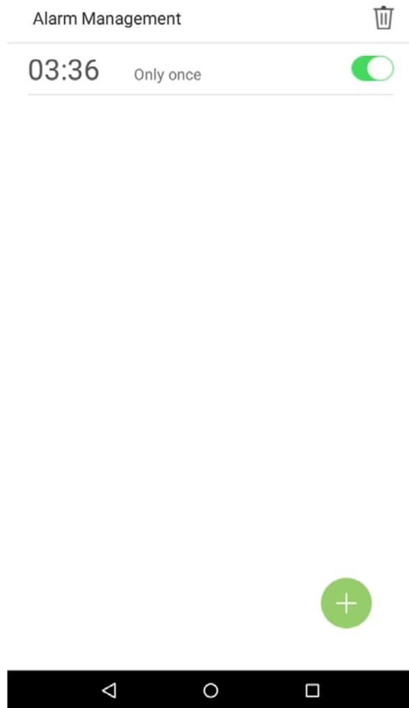
6. Enable [Alarm Switch] to change the alarm's status. Green indicates that the alarm is on, while gray indicates that the alarm is off.
