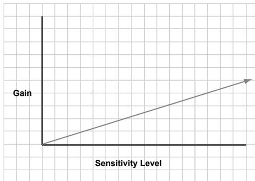
Figure 5-3: Gain adjustment principle
