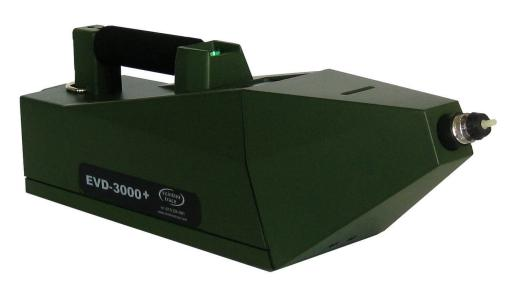
The handheld EVD-3000+ detects trace amounts plastic and high vaporpressure explosives, including C-4, PETN, Semtex, RDX and nitroglycerine. Using thermo-redox technology, the system can analyze either trace or vapor samples and delivers clear results in less than 10 seconds with the push of a button. No carrier gas or radioactive source is needed to operate the system, increasing safety and reducing ownership costs.
